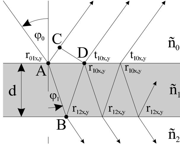
Figure 1.3: Interference in an ambient/film/substrate system
