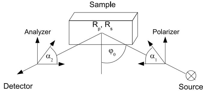
Figure 1.1: Schematic setup of an ellipsometer.  $R_p$ ,  $R_s$ : complex reflection coefficients for parallel and perpendicular component, respectively;  $\alpha_1$ ,  $\alpha_2$ : angle of the polarizer and analyzer;  $\phi_0$ : angle of incidence.
