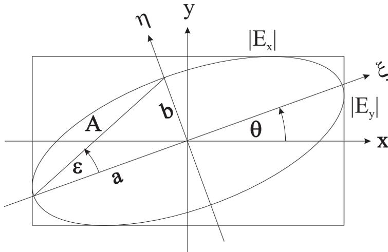
Figure 1.2: Parameters determining the Polarization Ellipse: Azimuth angle  $\Theta$ , amplitude  $A$  and ellipticity  $\tan \epsilon = b/a$ . The time dependence of the electric field vector can be described by superposition of two linearly, along the coordinate axis polarized orthogonal waves  $E_x(\vec{r}, t)$  and  $E_y(\vec{r}, t)$ .
