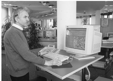
Figure 1.2: An ADAC dispatcher at work. The computer system registers via GPS the exact position of the service units at any time. Information about emerging help requests is received by phone from the call centers. Orders are transmitted to the units over radio. (Taken from ADAC's press office).
