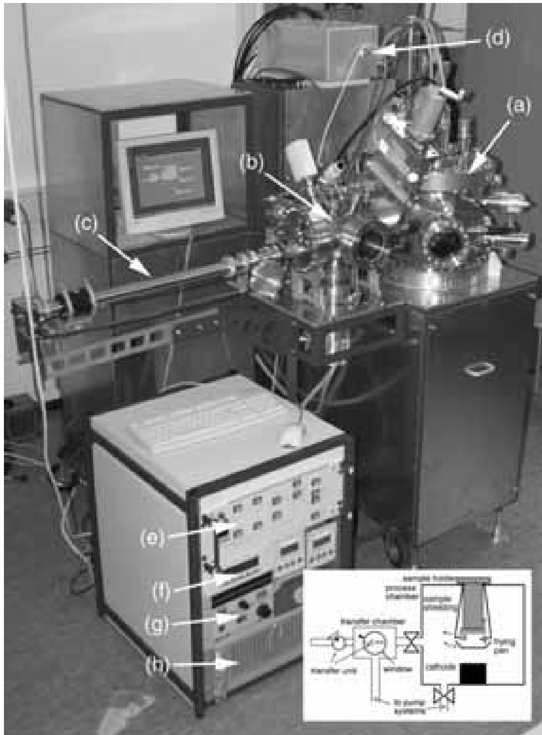
Figure 2.3: Photograph of the UHV sputter system for ferromagnetic materials. The inset shows a schematic of the system. (a) Process chamber, (b) Transfer chamber, (c) Transfer unit, (d) Matchbox, (e) Main electronics, (f) Pump and vacuum sensor readout, (g) DC and ac power supplies, (h) Process control computer.
