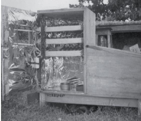
**Fig. 1: Solar Incubator**
