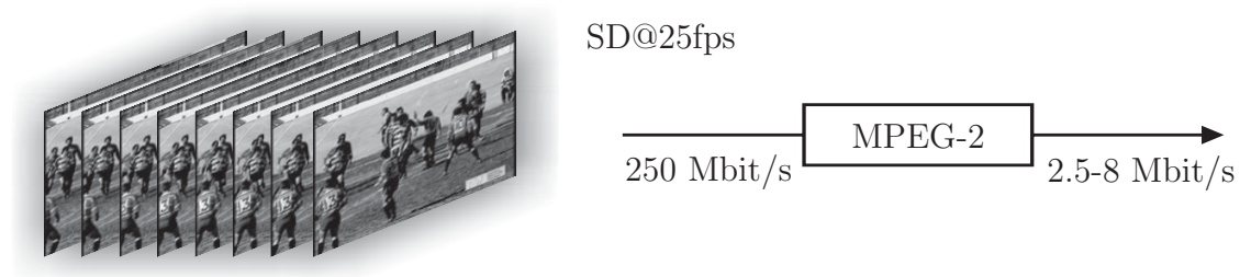
Figure 2.3: Typical video characteristics of stationary TV signals
