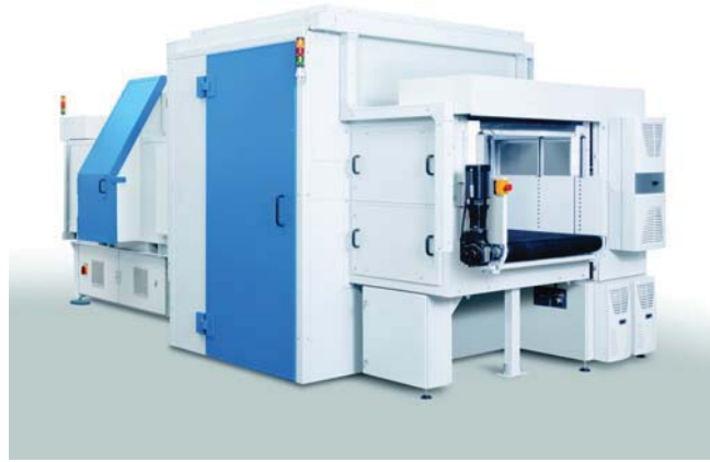
Figure 1.1: The baggage screening system GE XRD 3500 TM is fully automated and TSA certified. Image courtesy GE Security Germany GmbH.
