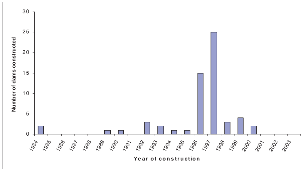
Figure 2.1: Number of micro-dams constructed in Tigray, N. Ethiopia by year. The dams' capacities range from 3.10 \cdot 10^6 \text{ m}^3 to 0.11 \cdot 10^6 \text{ m}^3 and a height of 9 to 24 meters. In an international context, the dams can be classified as small to medium size 3 (Source: CoSaERT unpublished reports)
