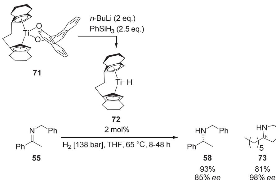
**Scheme 19:** Titanocene **72** catalysed asymmetric hydrogenation of imine **55**
