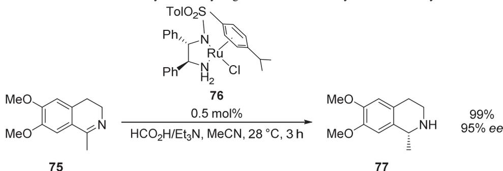
**Scheme 21:** Asymmetric hydrogenation of tetrahydroquinoline **75** by ruthenium catalyst **76**
