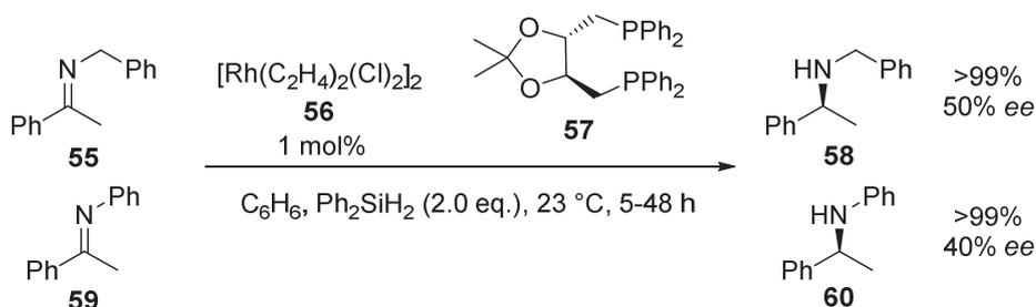
**Scheme 13:** Asymmetric rhodium-catalysed imine hydrosilylation of **55** and **59**
