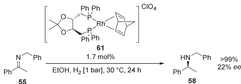
**Scheme 14:** Asymmetric rhodium-catalysed imine hydrogenation of **55** using **61**
