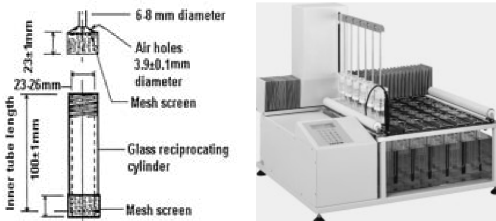
Figure 1.3.2 USP apparatus III, reciprocating cylinder, BioDis
