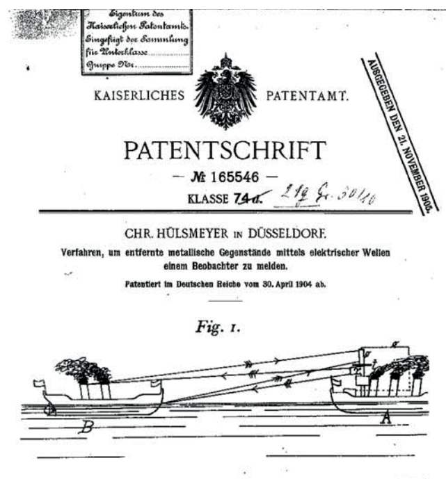
Figure 1.1: Hülsmeier's patent of the first radar, called "Telebiloskop"
