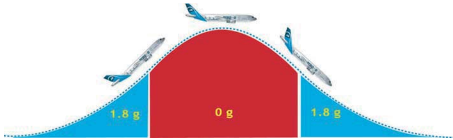
Figure 1.2: Natural gravity ranges in one parabola of a parabolic flight. Each parabolic flight consists of 31 parabolas. Courtesy of Novespace (2012)
