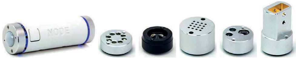
Figure 1.4: VARIABLE NODE+ with some of the available exchangeable sensor plugs.
