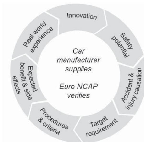
**Figure 4: The “Beyond NCAP” methodology requires that the vehicle manufacturer presents a detailed step-by-step analysis of the innovation’s potential safety impact, based on accident data and test results**
