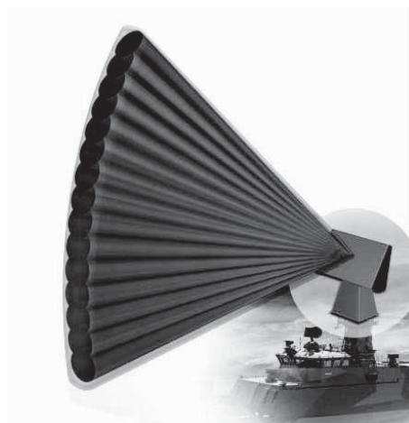
Figure 4. Multiple Beams on Receive
