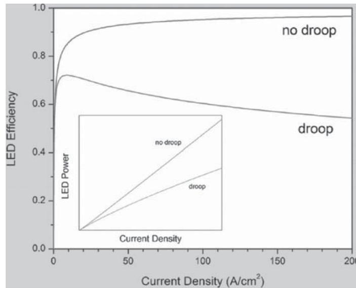
**Figure 1.3:** Illustration of LED efficiency droop (simulated). [24]
