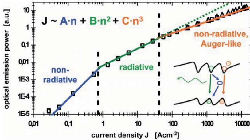
**Figure 1.4:** Emission power versus current density for a green-emitting multi-QW (MQW) LED. Different slopes can be attributed to different terms dominating the recombination-rate equation (e.g., solid blue, green, and orange lines). The corresponding recombination processes are shown in the band-diagram inset using the same colors. [41]
