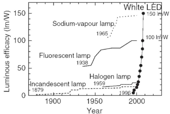
**Figure 1.1:** The history of luminous efficacy in incandescent lamps, halogen lamps, fluorescent lamps, sodium-vapour lamps and commercial white LEDs. The development years of white light sources are also shown. [20]
