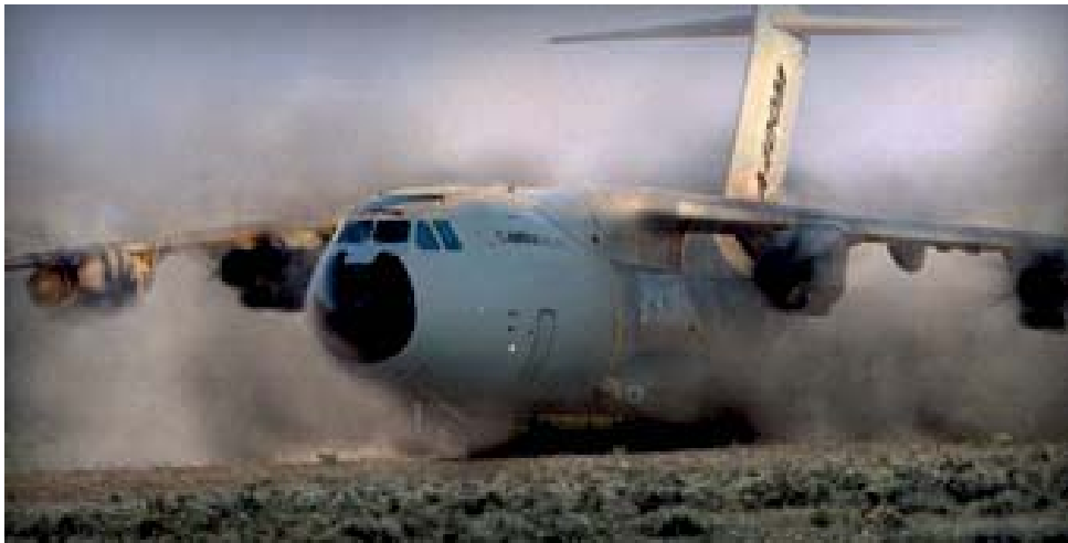
Figure 1.1: Landing of aircrafts in dusty environments leading to erosion of components (Reference: Airbus)
