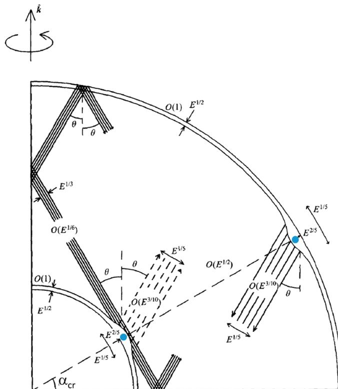
**Figure 1.4:** Velocity field and length scale in orders of the Ekman number of internal shear layers in a rotating spherical shell, where the background velocity field is  $O(Ek^{1/2})$ . The bulge at the inner and outer denotes the critical latitude (figure from Kerswell (1995)).
