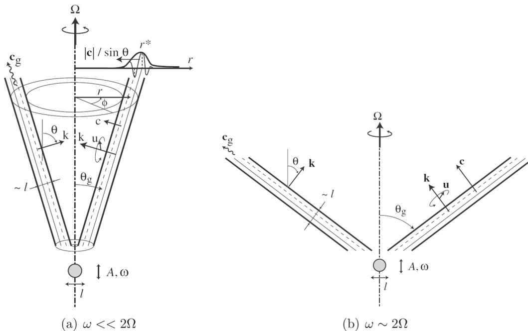
**Figure 1.2:** Sketch of the cones of inertial waves with increasing frequency  $\omega$ . Both are forced by oscillating disturbance of size  $l$  a and show the upper half cone. Trough and crest in the conical wave packet are illustrated as solid and dashed lines. a) A small oscillation much lower than  $2\Omega$  b) Stronger forcing nearly up to angular velocity  $2\Omega$ . (Messio et al., 2008)
