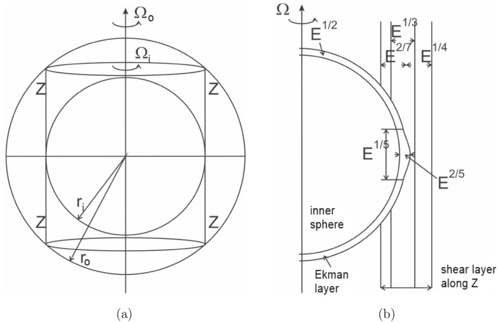
**Figure 1.3:** Stewartson layer in differential rotating spherical shell: a) cylindrical shear layer formation tangential to the inner sphere along  $Z$ , b) separated Ekman layers with their different widths (after Stewartson (1966)).
