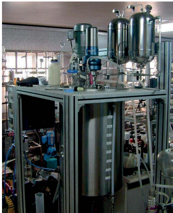
Figure 1: Reactor for conversion of rubber seed oil into FAME.
