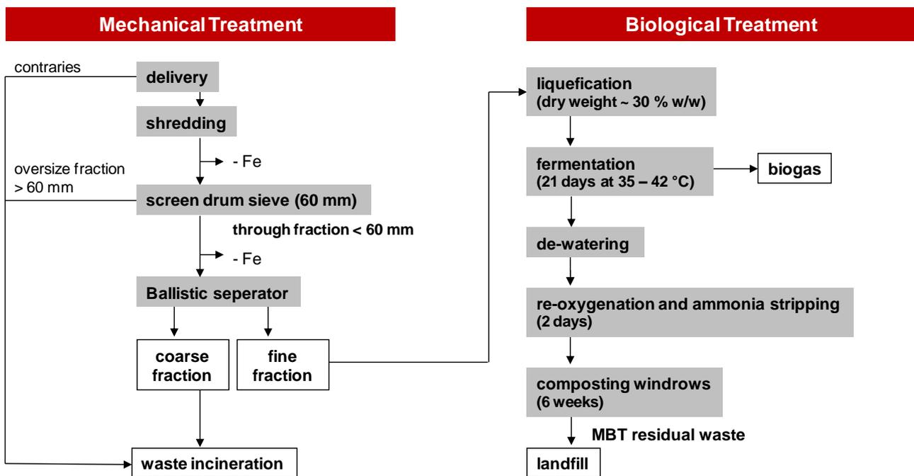
Figure 1-1: Schematic process in MBT plant in Hanover [16].
