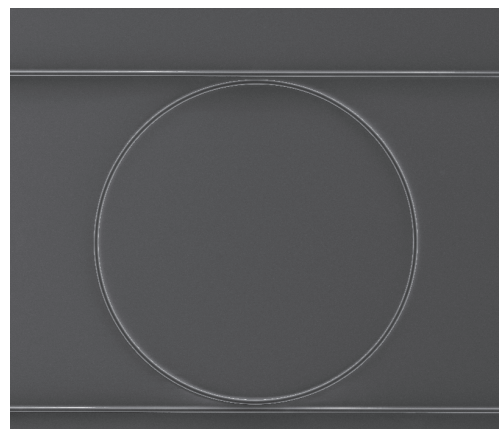
Figure 1: SEM image of a ring resonator with adjacent waveguides.
